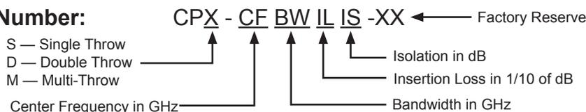
Example: To order a SPDT switch with center frequency of 60 GHz, 4 GHz bandwidth, 2.2 dB insertion loss and 20 dB isolation, specify CPS-60042220-XX.
